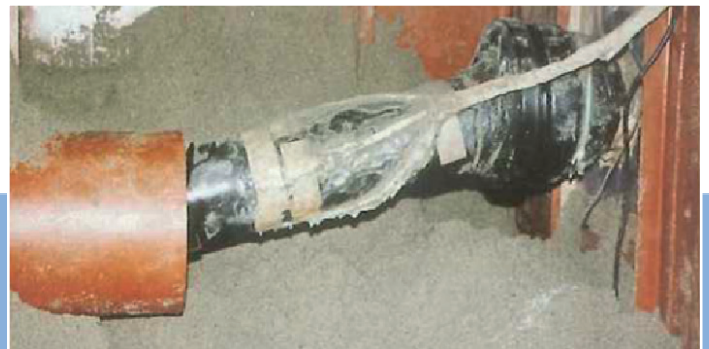
Test bed designed to recreate seismic earth movements: GEOFLEX® DN 150 - Deflection 200mm
